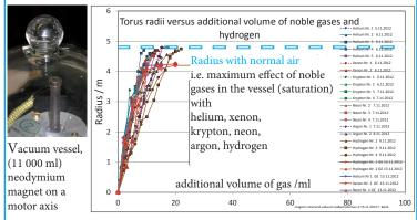
A bar magnet in an evacuated chamber rotates with constant velocity. The size of the outermost shell of the structure depends on the added volume of noble gases. Above a certain pressure, saturation of the radius results.<sup>2</sup>
