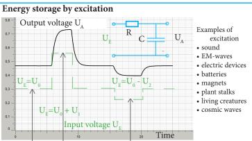
Time dependence: analogous to the output voltage of a low-pass filter.
