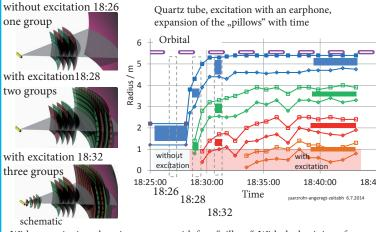
Without excitation, there is one group with four "pillows". With the begining of exitation, by an eletrically driven earphone, more groups arise, and the pillows move to the outermost shell.
