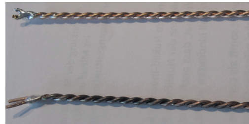
Figure 53: Above: Two copper wires (cross-sectional area: 1.5 \text{ mm}^2 ) have been twisted with the vise and power turn-screw. They have been soft-soldered at the ends. The material is highly deformed. Below: After the same treatment, the wires have subsequently been soft-annealed in a flame. (The surfaces of the wires are tarnished.)
