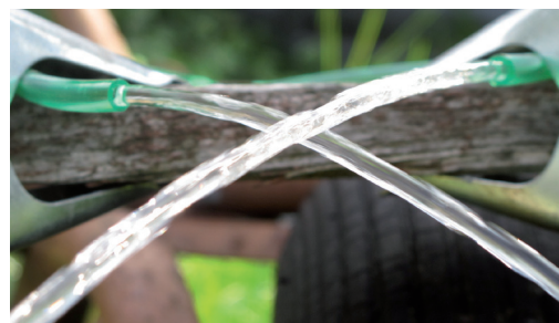
Figure 08 and figure 09: Two jets of water crossing askew: Air is entrained by the jets of water. At the crossing point, vortices are formed, not only in the air; bbewegte-materie.htm#kapitel-03-03
