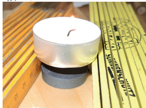
Figure 38: A candle is burning at some distance over a permanent magnet. This experiment should be performed only briefly!
