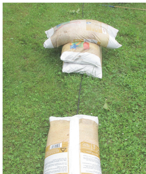
Figure 22: A black water hose is placed under sand bags, whose purpose is to simulate ground strata with an adjustable cover.
