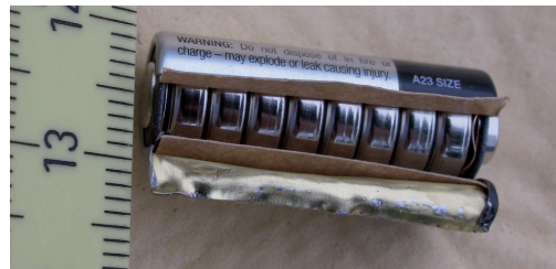
Figure 34: This 12 volt A23 battery consists of eight button cells connected in series ( 8 \times 1.5 \text{ V} = 12 \text{ V} ). batterien.htm
