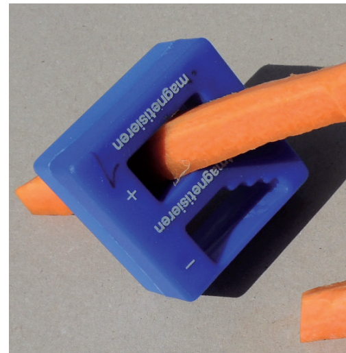
Figure 47: A "magnetiser-demagnetiser" or "degausser" is available at about 4 Euro from an electronics supplier. With the use of this device, the perceptible structures associated with a plant section can be varied. This device is normally employed for magnetising or demagnetising tools, such as screwdrivers.
