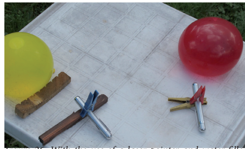
Figure 26: With the use of a laser pointer and water-filled balloons, the laser beam can be directed toward the water either centrally or tangentially. Yellow: The laser beam is directed toward the right-hand edge. Red: The laser beam is directed toward the left-hand edge.
