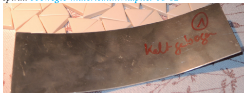
Figure 57: Aluminium sheet, bent in the cold condition
