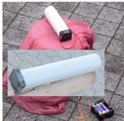
Figure 40: A small computer fan is installed in a thick cardboard mailing tube and blows air through the tube. Instead of the usual operating voltage of 12 V, it is supplied with only 4.5 V from three 1.5 V flashlight cells. eenergiesparlampe-gewendelt.htm#kapitel-06 kuehlwasser-zwanzig.htm#kapitel-01-03
