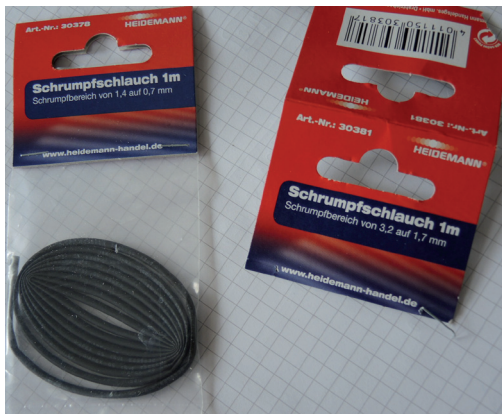
Figure 16: Shrink-fit hose is thermoplastic and contracts somewhat upon heating (shrinkage). This hose is well suited for experiments with flowing water.
