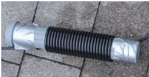
Figure 15: A thin water hose is wound as a coil on a sewer pipe. kuehlwasser-vier-05.htm
