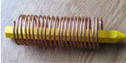
Figure 55: An uninsulated copper wire has been wound into a coil. Oil chalk is present in the interior of this coil.
