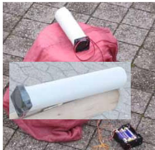
Figure 40: A small computer fan is installed in a thick cardboard mailing tube and blows air through the tube. Instead of the usual operating voltage of 12 V, it is supplied with only 4.5 V from three 1.5 V flashlight cells.
