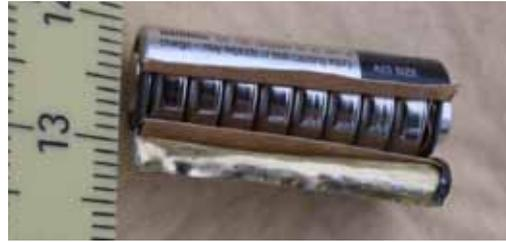
Figure 34: This 12 volt A23 battery consists of eight button cells connected in series ( $8 * 1.5 \text{ V} = 12 \text{ V}$ ). [batterien.htm](#)
