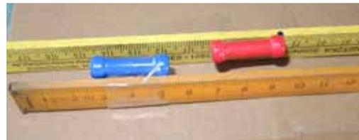
Figure 31: Each magnet has been pasted to the end of a metre stick for easier manipulation. Thus, the magnets can also be more easily forced into a position with like poles together.
