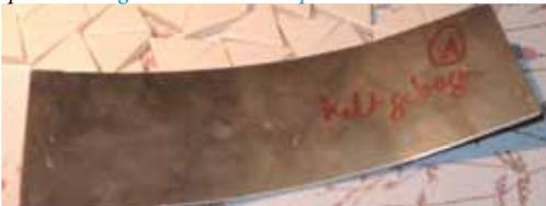
Figure 57: Aluminium sheet, bent in the cold condition
