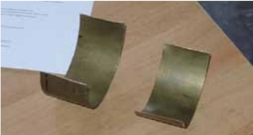
Figure 58: A brass pipe has been sawn into two sections. After the sawing process, the pipe has expanded diametrically. Evidently, mechanical stress was still present in the pipe, as a result of the drawing process during manufacture. [strom-sehen-011.htm#kapitel-11](http://strom-sehen-011.htm#kapitel-11)
