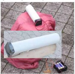
Figure 40: A small computer fan is installed in a thick cardboard mailing tube and blows air through the tube. Instead of the usual operating voltage of 12 V, it is supplied with only 4.5 V from three 1.5 V flashlight cells.
