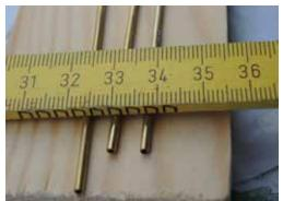
Figure 21: The small-diameter brass pipe is available from a building-supply store (diameter of bore: 1 mm).
