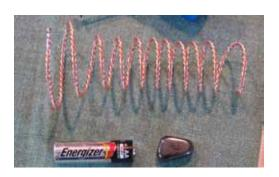
Figure 54: The twisted copper wire has been wound around the neck of a wine bottle. If a flashlight cell or a permanent magnet moves along its longitudinal axis (for instance, by allowing it to fall through the coil), the perceptible properties of this coil vary.
