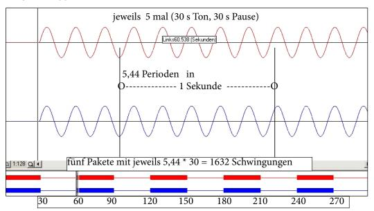
Figure 25: This "music" file can be "played" on the thin water pipe: five packets each 30 s sound and 30 s pause, at 5.44 Hz; program: Creative WaveStudio 6.01, (Freeware); above: section (3 seconds), below: 300 seconds total time, file: dvt\_b035-5-44hz-mit-pausen.mp3
