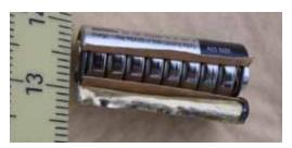
Figure 34: This 12 volt A23 battery consists of eight button cells connected in series (8  $\times$  1.5 V = 12 V). batterien.htm
