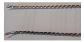
Figure 53: Above: Two copper wires (cross-sectional area: 1.5 mm²) have been twisted with the vise and power turn-screw. They have been soft-soldered at the ends. The material is highly deformed. Below: After the same treatment, the wires have subsequently been soft-annealed in a flame. (The surfaces of the wires are tarnished.)
